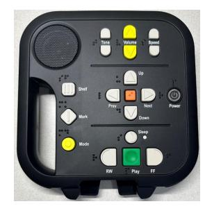
Image is of a square, black talking book machine, with a handle on the left side, underneath the speaker. Alongside the handle are buttons for Shelf (square), Mark (diamond), and Mode (Round, yellow).
